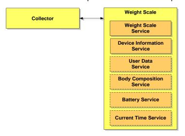
Notes: Profile roles (Collector, Weight Scale) are represented by yellow boxes and services (Weight Scale Service, Device Information Service, Body Composition Service, User Data Service, Battery Service and Current Time Service) are represented by orange boxes.
